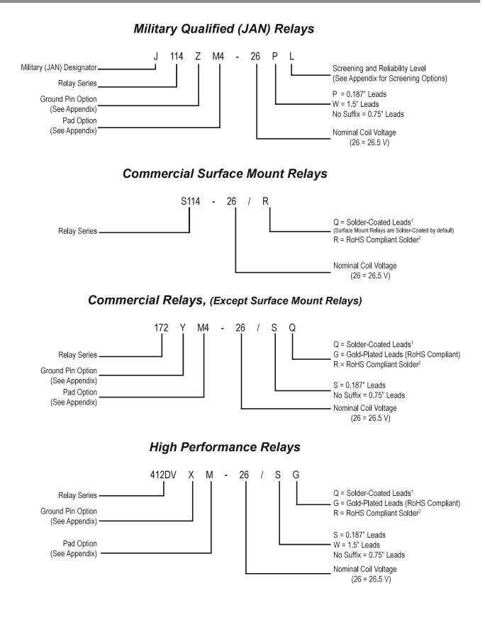
General Note: Parts ordered without suffix may be supplied with Solder-Coated or Gold-Plated leads. 1 Parts ordered with Solder-Coated leads will have (Sn60/Pb40) 2 Parts ordered with RoHS Solder-Coated leads will have (Sn99.3/Cu0.7)
